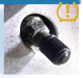
Dill's USA-Made 5010 TPMS Hex Nut Removal Kit is the only safe way to remove a seized TPMS valve stem.
